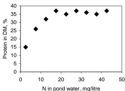
**Figure 10:** Protein yield through a one year cycle from duckweed grown in ponds fertilized with biodigester effluent (Source: Nguyen Kim Khang 2000)
